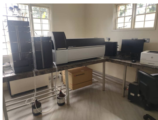
Figure 14: High-performance liquid chromatograph-triple quadrupole mass spectrometer (LC/MS/MS) at the Biomarker Discovery lab, Kasangati
