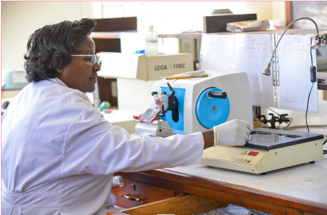
Researcher conducting histological analysis in the Pathology Laboratory supported by MakBRC, utilizing the Leica 1150C Microtome for precision tissue sectioning. This essential equipment enables detailed examination of biological samples, contributing to diagnostic and research efforts in pathology and biomedical sciences.
