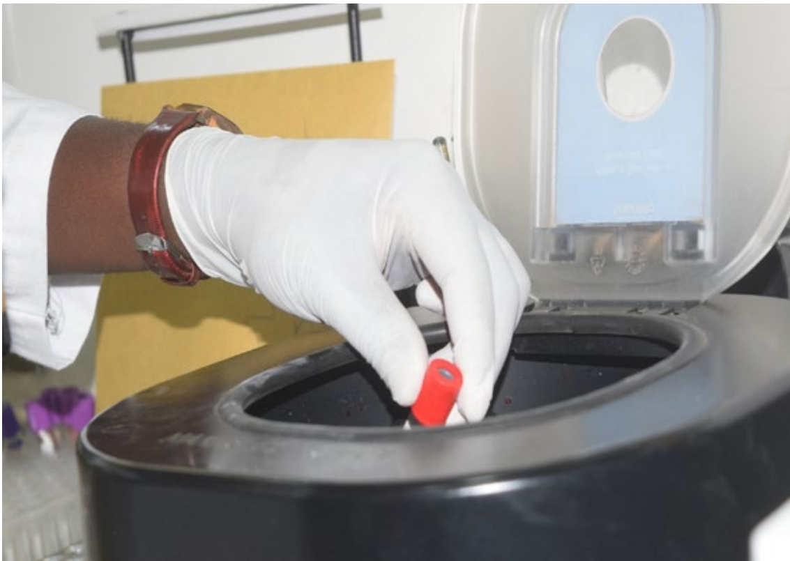
Refrigerated Centrifuge machine it separates the specimens into liquid and solid parts
