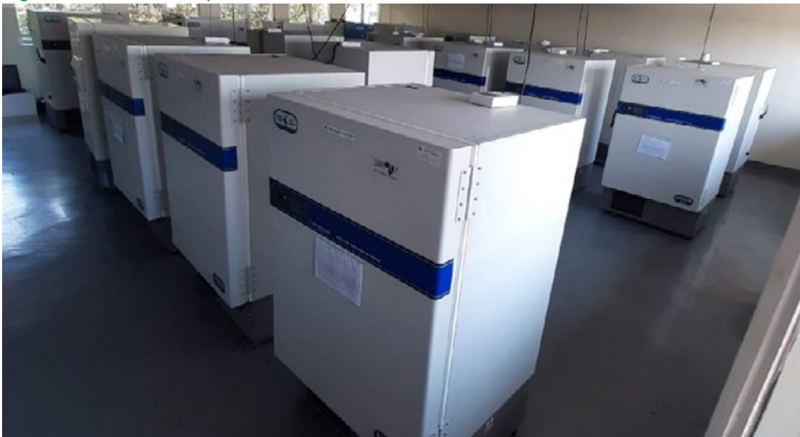
ULTRA freezar used for sample storage for a period of time
